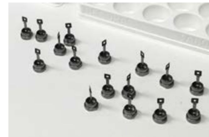
Fig. 4 Polymer supports mounted on pins fitting to the sample-changing robot. The area of the perforated 2 \mu\text{m} thick polymer film is 2x2 mm 2 in size, suspended in a 5x5 mm 2 sized frame.
