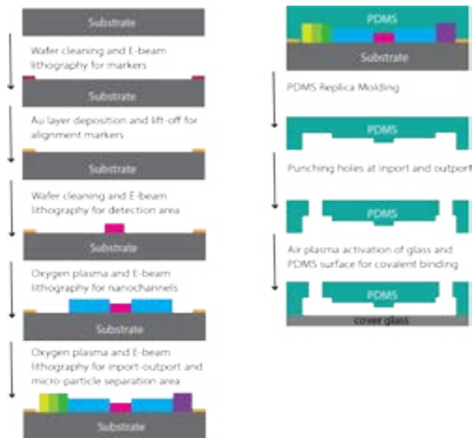
Fig. 1 Fabrication and development of lab-on-a-chip platform using state of art lithography processes on a Si wafer and replica molding using polydimethylsiloxane (PDMS). The final integrated micro/nanofluidic device was developed using air plasma activation of patterned PDMS and a cover glass.
