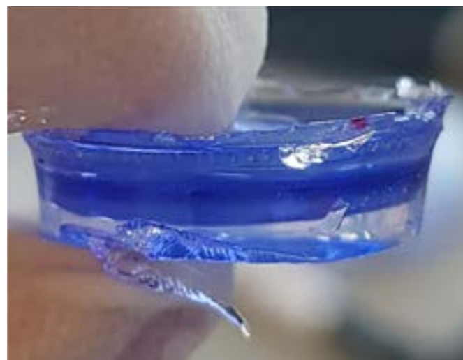
Fig.1. Blue colored layers with variable crosslinking degree.
