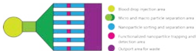
Fig. 2 Schematics of a lab-on-a-chip platform for early disease detection using antibody-functionalized nanoparticles. The blood sample is injected at the in-port area in combination with functionalized nanoparticles allowing antibody-antigen binding on the nanoparticle surface, and detection of bound antibodies at the detection area.
