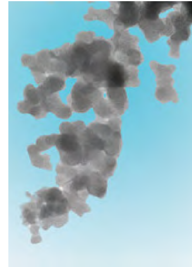
In the Nano Argovia project SiNPFood, methods for characterizing silicon oxide nanoparticles (SiNPs) are being investigated. (Image: FHNW)
