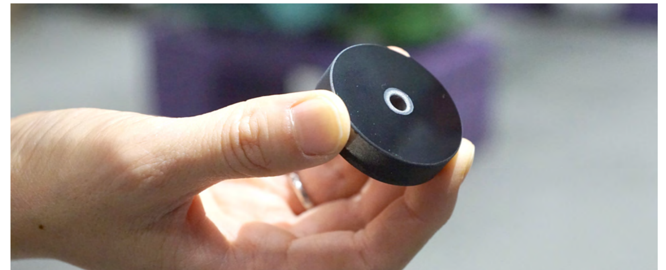
The samples were coated with a ceramic layer using the plasma spray method, which is then closely examined and post-treated.
