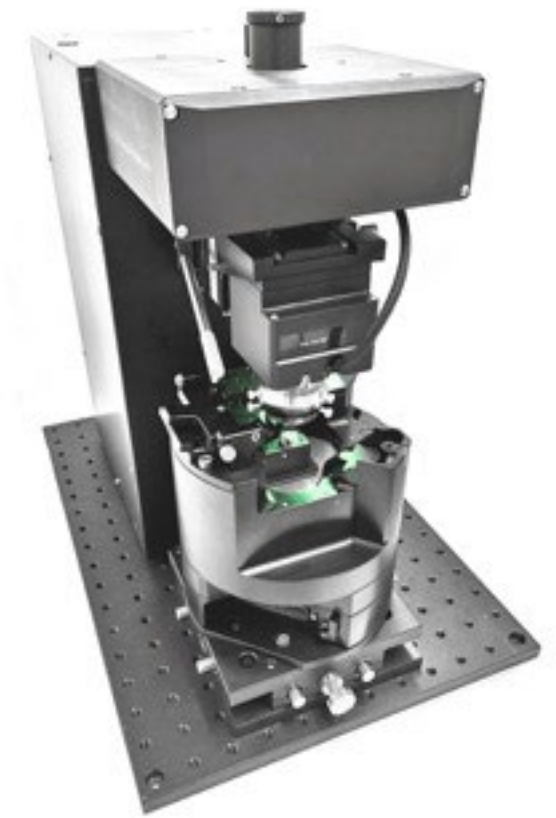
The NQsense project helped Qnami to present the ProteusQ – the first commercial quantum platform for material analysis at nanometer resolution – at the end of 2019. (Image: Qnami)
